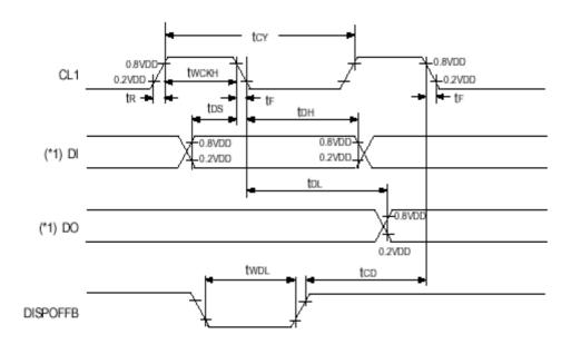
(\*1) When in single-type interface mode  $DI \Rightarrow D2\_DL(SHL="L"), D4\_DR(SHL="H")$   $DO \Rightarrow D4\_DR(SHL="L"), D2\_DL(SHL="H")$ When in dual-type interface mode  $DI \Rightarrow D2\_DL$  and  $D3\_DM(SHL="L"), D4\_DR$  and  $D3\_DM(SHL="H")$  $DO \Rightarrow D4\_DR(SHL="L"), D2\_DL(SHL="H")$
