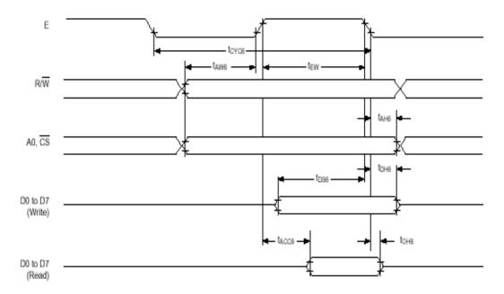
Note: toyos indicates the interval during which CS is LOW and E is HIGH.
