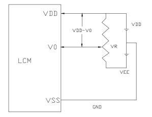
Vdd-V0: LCD Driving Voltage
